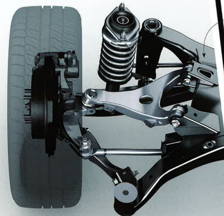
Front: suspension layout is from the Subaru STi but the new engine mount requires the lower arm to be reversed
