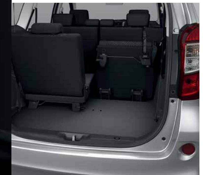
Second row seats split forward for easy access to the rear, while the third row split-seat, cushion-tumble feature enables expansion of the luggage space.
